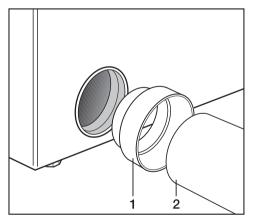
The Miele adapter (1) is inserted onto the vent opening on the dryer.
